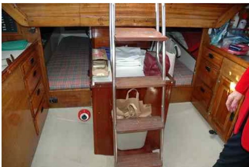
This photo show the new engine box and ladder. The top of the engine box is Formica and adds storage but can be removed and the entire box lifted off to allow access to the engine. The top step of the ladder is wider to keep grandchildren from falling through.
