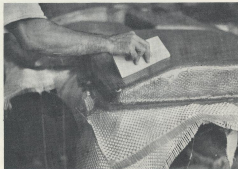
Careful squeegeeing of each lamination yields a high-density layup.
