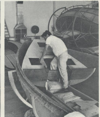
The wooden interior is installed while the layup is still in the mold, preventing any distortion of the hull contours.
