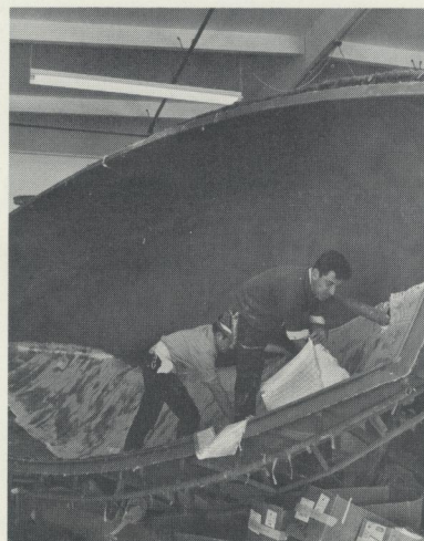
As resin is applied the new lamination becomes a permanent part of the hull.
