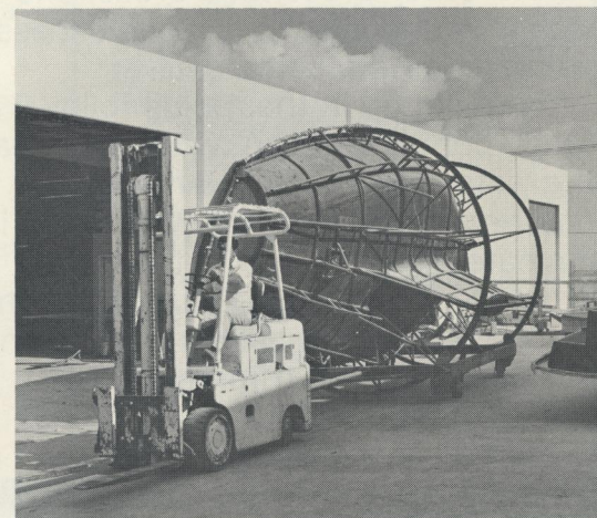
An elaborate steel framework holds every contour of the mold rigidly in place.
