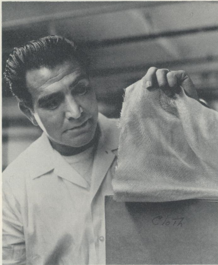
Glass cloth is a loose weave of twisted strands of glass fiber—weight depends on the size of the strands.
