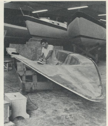
The reinforced topside layup is sanded smooth before painting.
