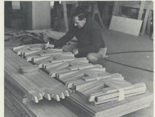
Boat interiors start with precut parts in the Wood Department.
